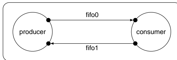
Figure 2.3: Modified Producer-Consumer example suffering from deadlock.
